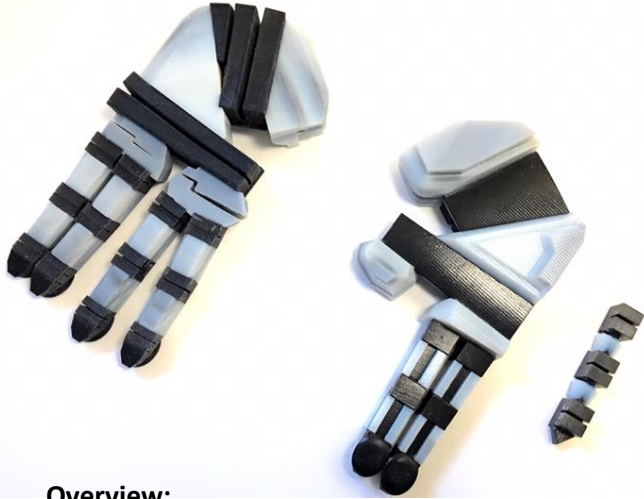
From left to right: Modular version of gripper, first print of palm with two fingers, early finger prototype
